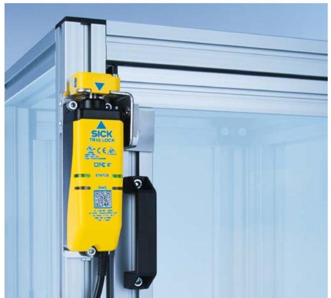
The movable physical guard is locked with a maximum locking force of 1,690 N, the semiconductor outputs (OSSDs) are switched on.
