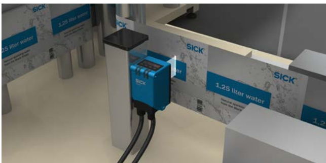
Detecting cutting positions.
