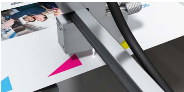
Detecting registration marks on printing machines.
