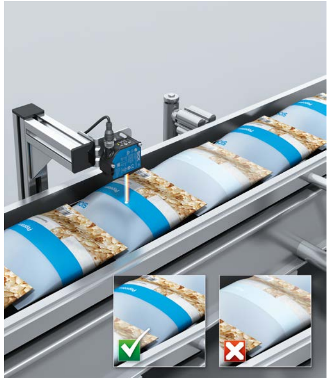
Detecting packaging with faulty printing.
