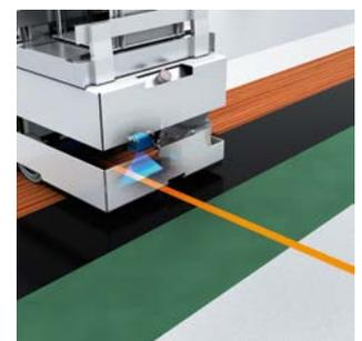
The OLS detects the luminescent line regardless of the physical features of the floor and background. A separate teach-in process is not necessary.
