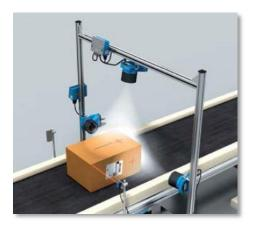
example, a 1024 x 768 pixel sensor captures a rectangle-shaped image at that resolution. The camera takes multiple pictures, capturing anywhere from five to 100+ images per second, depending on the capabilities and actual resolution of the individual device. The images are decoded by the camera, which transmits the information to upper level control systems.
