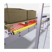
pallet by looking for two to five objects that are no larger than 240 mm in size. Once it has determined that the number and the size of the objects are consistent with a pallet, it allows the pallet to pass through—as long as the objects do not change in size and they remain a consistent distance apart.
