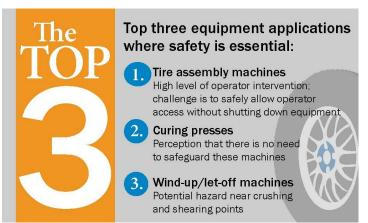
1. Consider tire assembly machines. Because of the level of operator intervention and number of moving parts involved, tire assembly machines are particularly hazardous. The operator is in and out of the process many times, and sometimes needs to be engaged with the machine while it is still moving. For example, a drum spins and wraps a ply onto it; when the drum comes around, it should make a perfect
