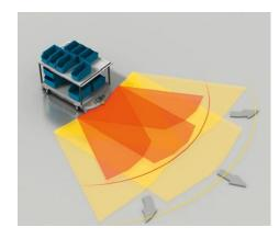
In addition, the size and design of the application will determine the ideal scanner size to use. The right size safety laser scanner helps ensure a streamlined looking machine and minimal costs and related downtime, due to damage, for end users.
