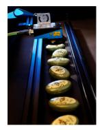
of the output. A blob tool could be used to check for presence and a pattern tool could verify if it is indeed the correct label. This combination gives information that using just one tool does not.
