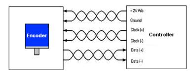
affect on the connectivity hardware, but it does need to match the specific SSI controller. The serial communication greatly reduced the wiring that was once required for position data, cutting costs and installation time.
