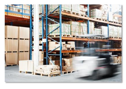
• OSHA standard 29 CFR 1910.178 (n)(4) for powered industrial trucks states: "If the load being carried obstructs forward view, the driver shall be required to travel with the load trailing." However, even though forklift drivers are trained to always look in the direction of travel (and to travel in reverse if the load blocks their view), they may not do so consistently.
