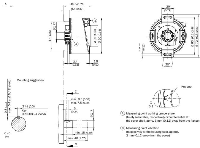
General tolerances as per DIN ISO 2768-mk Cable diameter =  $5.6 \pm 0.2$  mm; bend radius R = min. 7.5 x diameter cable
