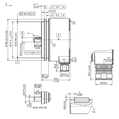
Solid shaft, servo flange, male connector connection, radial
