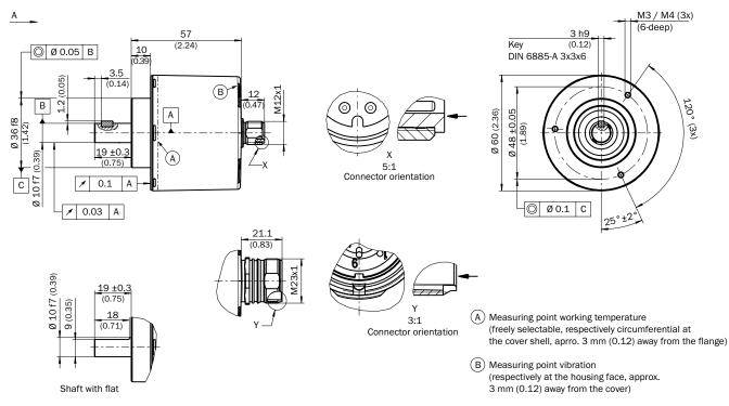
Solid shaft, face mount flange, male connector connection, axial
