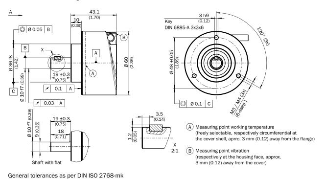
Solid shaft, face mount flange, cable connection
