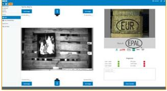
The PACS user interface displays the acquired images of the pallet's feet and load, an evaluation of the pallet type, and an indication of the probability for correct classification. PACS is easy to use. No programming knowledge is required.
