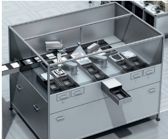
Figure 2: Cell stacking machines contain several grippers for stacking different materials.
