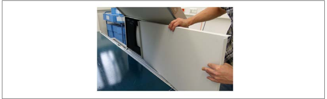
Fig. 76: Pulling the inner cover plate out of the reader module
