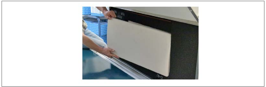
Fig. 79: Removing the antenna from the reader module
