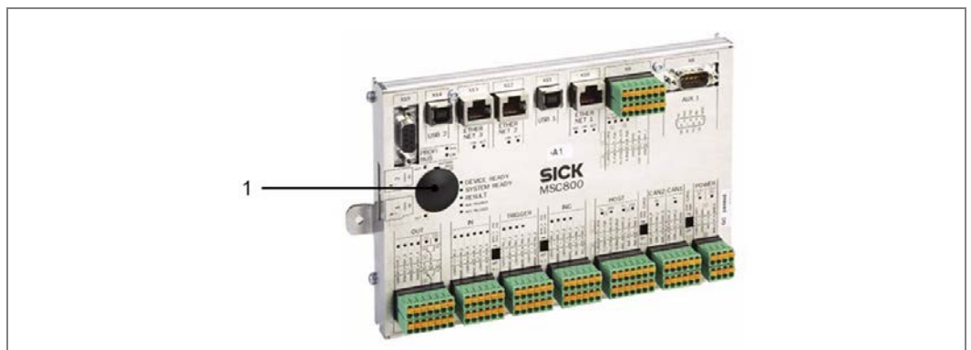
Fig. 67: Position of the battery in the MSC800 controller
