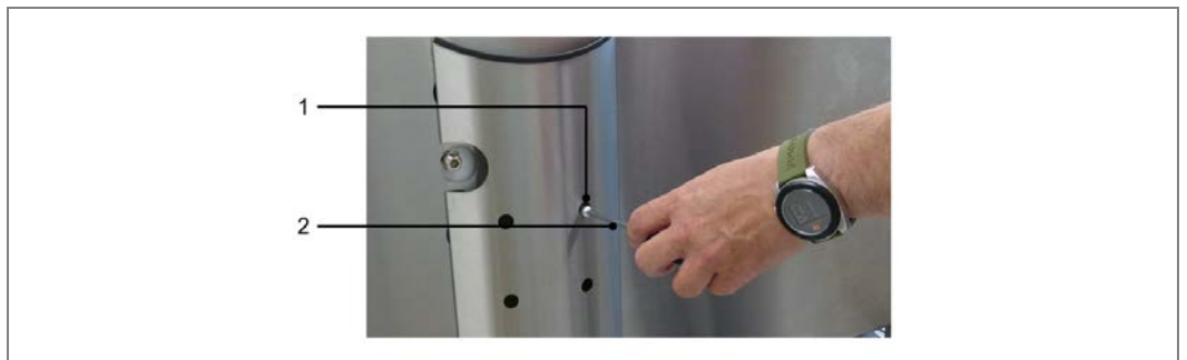
Fig. 78: Releasing the fixing nuts for the antenna
