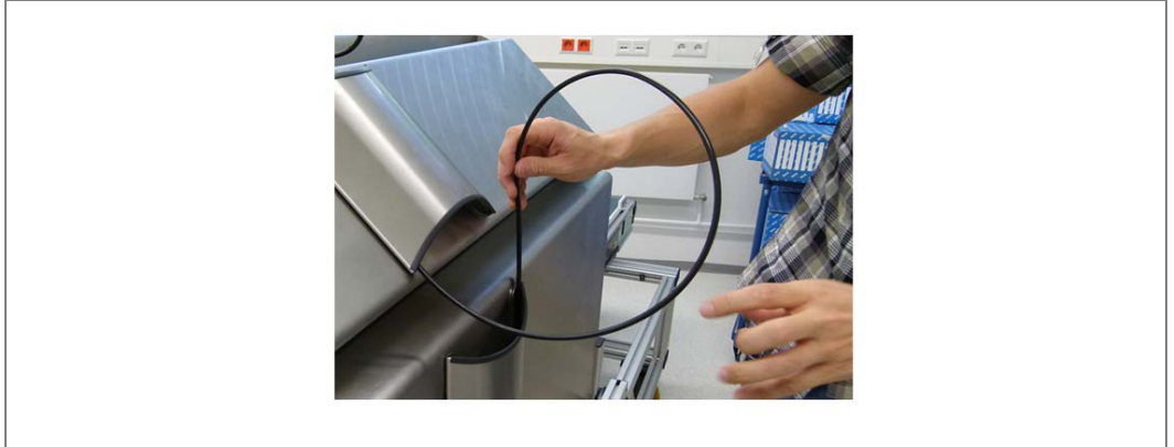
Fig. 54: Looping excess antenna download
