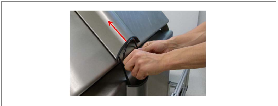
Fig. 55: Looping excess antenna download
