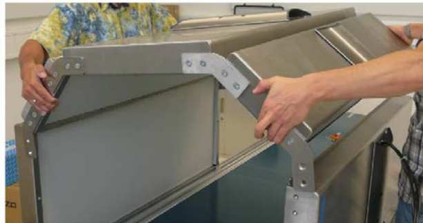
Fig. 23: Placing the group of modules on the side modules
