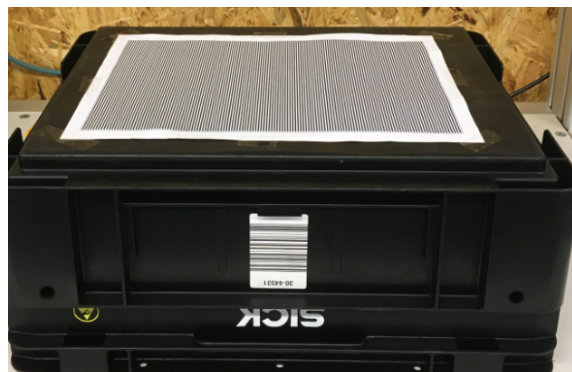
Fig. 11: Grid sheet for camera adjustment
