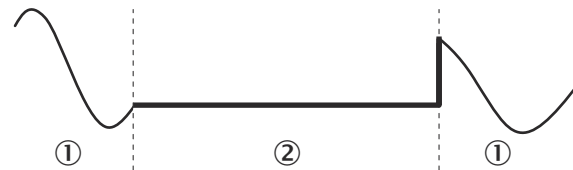
Figure 13: Hold alarm function
