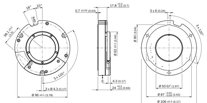
0 Measuring point for operating temperature
