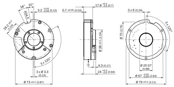
0 Measuring point for operating temperature
