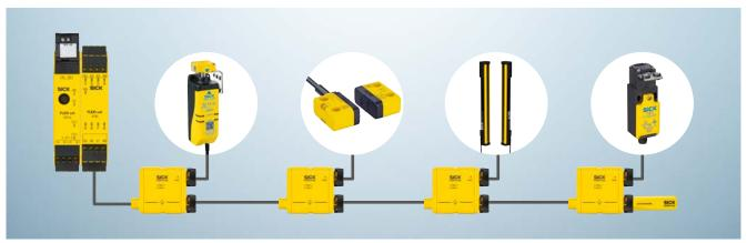
Safe series connection with Flexi Loop: up to 32 different sensors can be connected in series. Detailed diagnostics is possible using the Flexi Soft evaluation unit.
