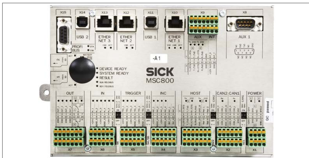
Fig. 22: MSC800-0000 logic unit in the cabinet of the MSC800-1100/-2100/-2300: position of the electrical connections
