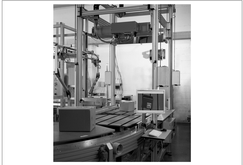
Fig. 7: MSC800 in combination with ID sensors for 1D / 2D codes on a conveyor system
