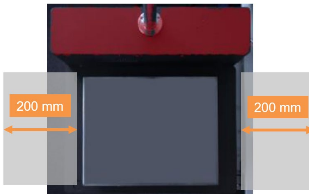
Fig. 77: Clearance on both sides of the scale
