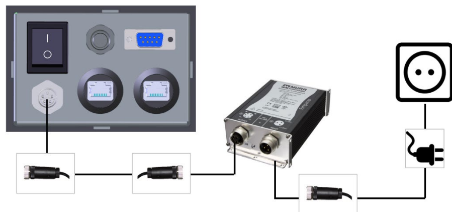
Fig. 40: Establishing connection to the voltage supply
