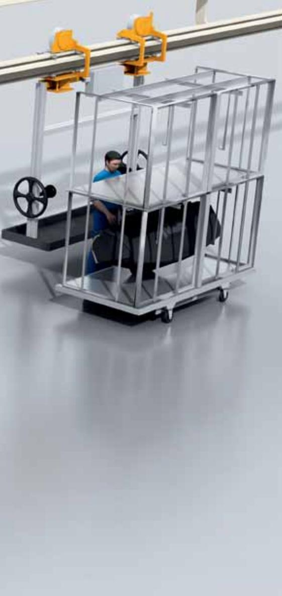
**Positioning the dashboard in the work station**
