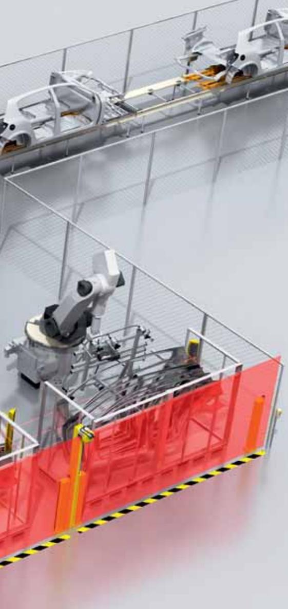
**Pick up of body in white parts for mounting**
