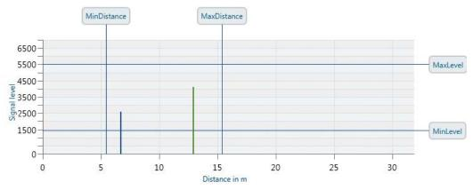
Fig. 4: Diagram defining the region of interest of the Dx1000 distance sensor from SICK.
