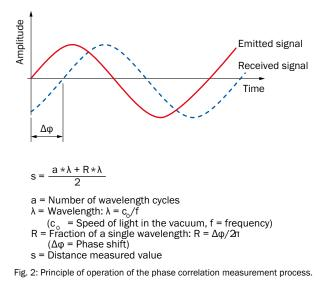
The phase correlation measurement process is particularly suitable for fast, high-precision distance measurement for objects that move continuously along the laser axis. This type of axial object tracking is used, for example, for determining the position of storage and retrieval systems in fully automated high-bay warehouses. The distance sensor usually moves with the storage and retrieval system and measures the distance to a fixed reflector at the end of the aisle.
