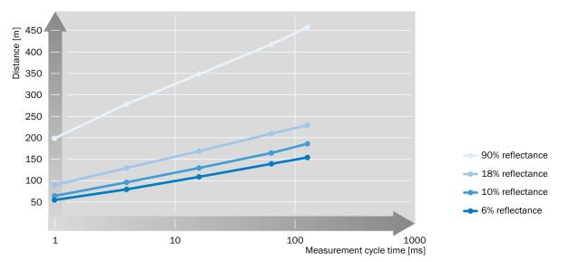
Fig. 7: By setting the measurement cycle time, the sensing range of the DT1000 distance sensor from SICK can be adapted to the respective application for measurements on natural target objects (i.e., not retro-reflective objects). The remission is an (object-dependent) measurement for the reflection of the measuring laser on the measuring object.
