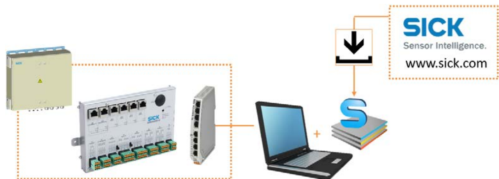
Fig. 63: Establishing the configuration PC – SIM2000-2 Prime controller connection
