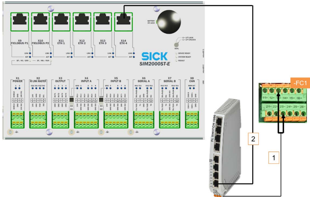
Fig. 57: Connection for LFT Ethernet switch (set up at the factory)
