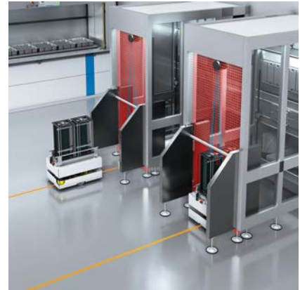
Hazardous area protection during AGV docking with the Safe Portal safety system
