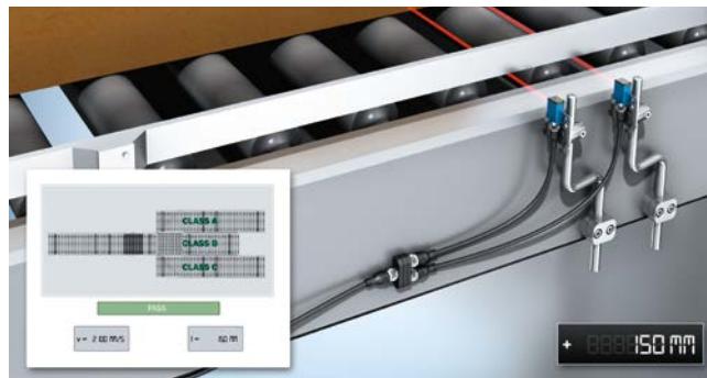
Fig. 7: Smart sensors as intelligent data collectors.
