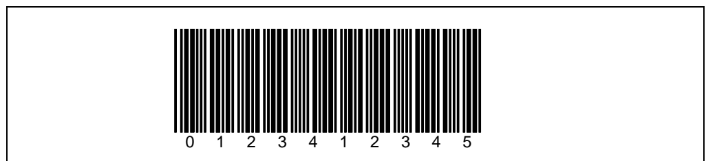
Fig. 6-1: Bar code pattern (code 39; module width 0.35 mm (13.8 mil); print ratio 2:1)
