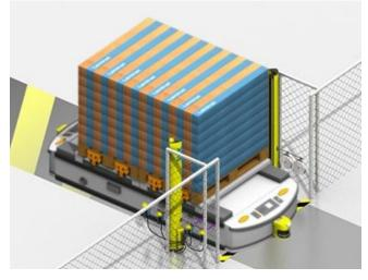
Entry/exit station with 4 muting sensors, the material can flow in both directions
