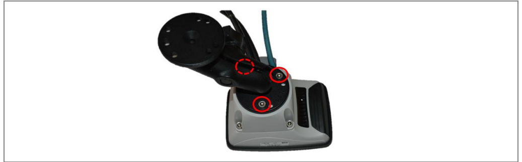
Fig. 48: Removing the operator display from the bracket
