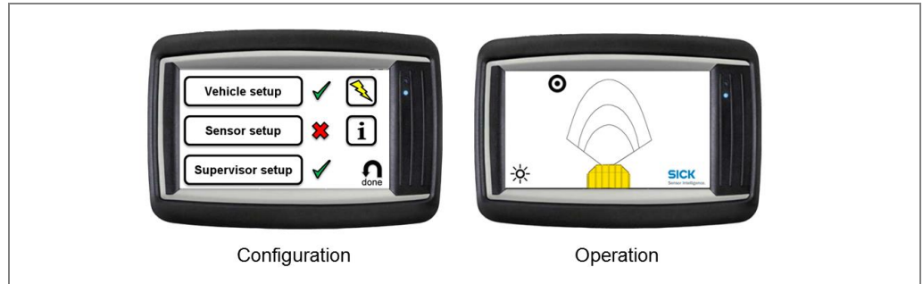
Fig. 14: The operator display in configuration and operating mode
