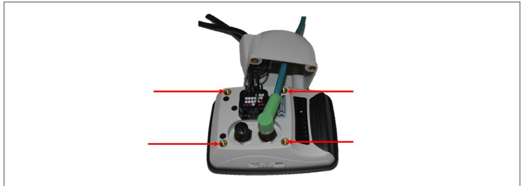
Fig. 49: Removing the adapter from the operator display
