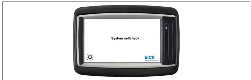
Fig. 43: Self-test of the system on the operator display
