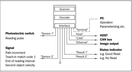
Fig. 3-2: Block diagram: functions of the ICR
