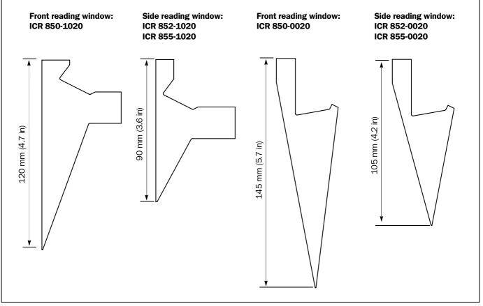
Fig. 4-6: Distance tools: assignment to the ICR types
