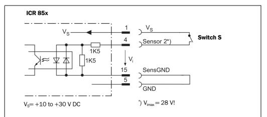
Fig. 10-13: "Sensor 2" configuration for triggering the teach-in match code 1
