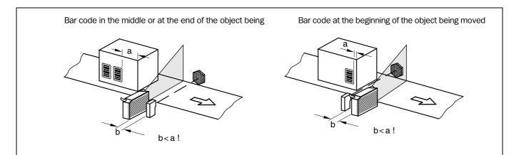
Fig. 4-12: Line scanner: Installation example for the external reading pulse sensor
