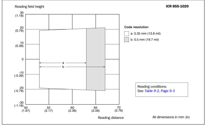
Fig. 9-4: ICR 855-1020: Reading ranges
