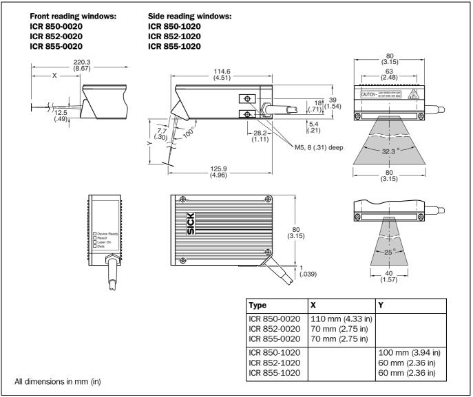
Fig. 9-1: Dimensions of the ICR
