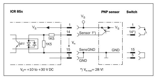
Fig. 5-5: Connections of the "Sensor 1" switching input
