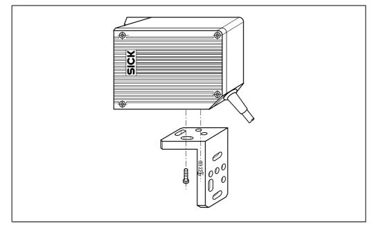
Fig. 4-3: ICR installation options using the mounting bracket no. 2 025 491
