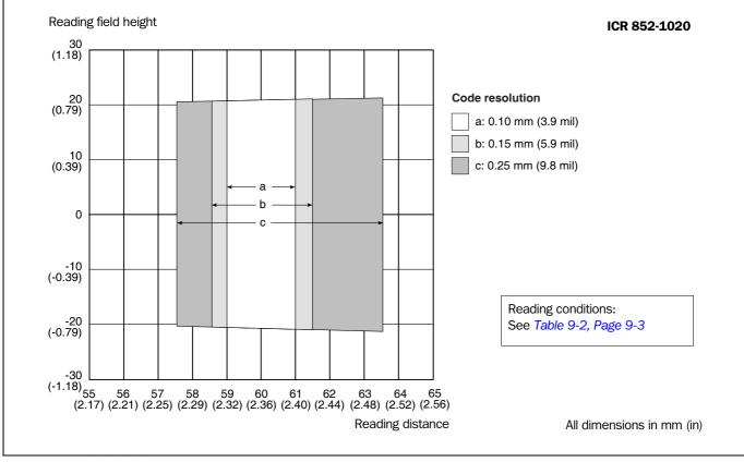
Fig. 9-3: ICR 852-1020: Reading ranges
