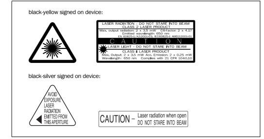
Fig. 2-1: Laser warning labels found on the ICR
