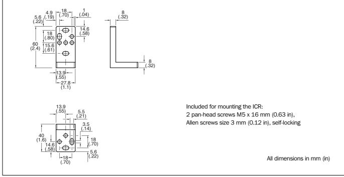
Fig. 10-16: Dimensions of the mounting bracket no. 2 025 491
