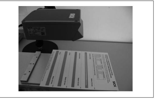
Fig. 6-8: Scanner adjustment: Adjusting the reading distance with the test pattern no. 8 010 754
