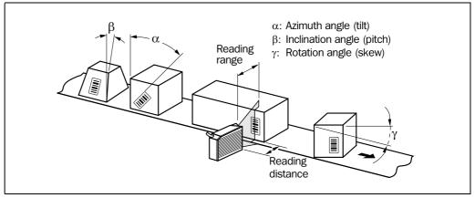
Fig. 4-8: Line scanner: Reading angles between the illumination line and the code
