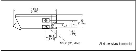
Fig. 4-2: Position of the securing threads on the ICR
