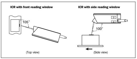
Fig. 4-9: Preventing surface reflection: Angle between the emitted light and code (tilted away from the vertical axis)
