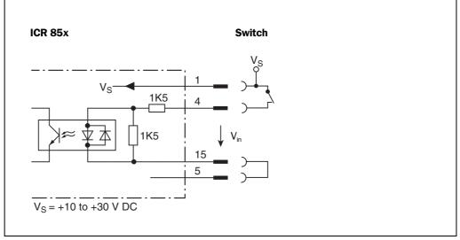
Fig. 5-6: Connections of the "Sensor 2" switching input
