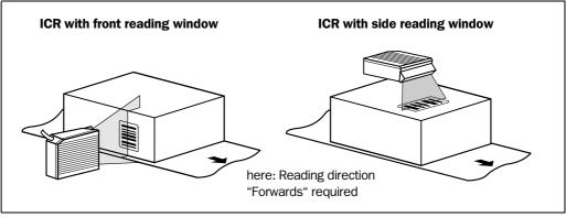
Fig. 4-4: Alignment of ICR with code and conveyor direction
