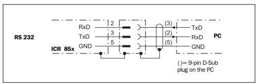
Fig. 5-4: Connection of the auxiliary interface
