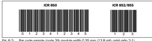
Bar code sample (code 39; module width 0.35 mm (13.8 mil); print ratio 2:1) Fig. 6-2:
