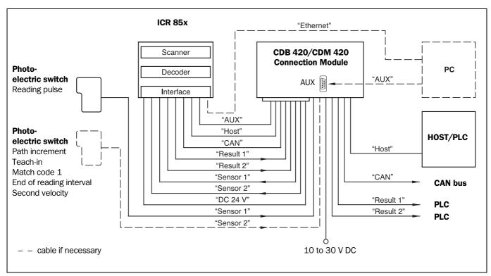
Fig. 5-1 shows the connection principle of the CDB 420 or CDM 420 for one ICR.
