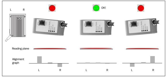
Fig. 6-10: Adjusting the ICR in the reading plane
