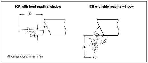
Fig. 4-5: Definition of the reading distance
