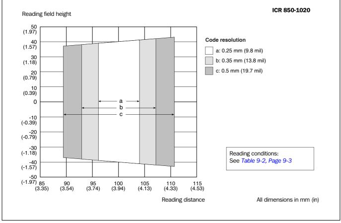
Fig. 9-2: ICR 850-1020: Reading ranges
