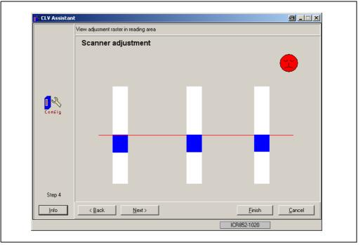
Fig. 6-9: CLV Assistant: "Scanner adjustment" dialog box
