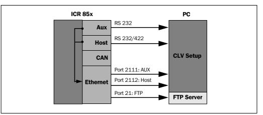
Fig. 5-3: Block diagram: Function of the Ethernet interface
