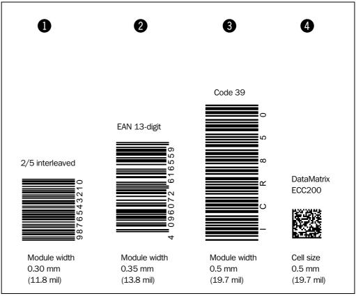
Fig. 10-18: Scannable 1-D codes with various module widths (print ratio 2:1)/2-D codes
