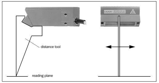
Fig. 4-11: Using the distance tool (in this example: ICR 85x with reading window on side)
