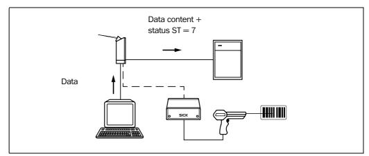
Fig. 10-14: Auxiliary input via the auxiliary interface of the ICR
