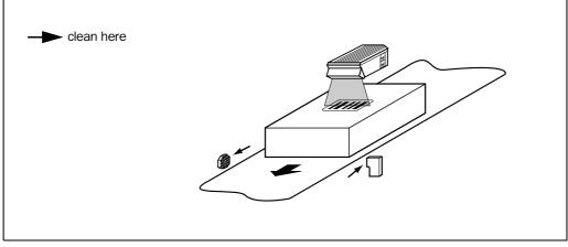
Fig. 7-2: Cleaning the external optical sensor (reading pulse generator)
