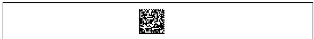
Fig. 6-1: 2-D code sample (DataMatrix ECC200; cell size 0.5 mm (19.7 mil))
