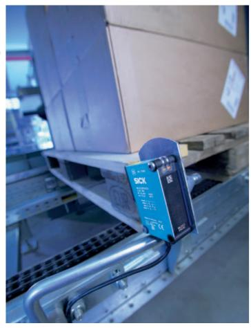
▼ Easy-Teach-in: Put energetic photoelectric proximity switch WTE23-2 quick and easily into function. Align on object, press Teach-in button 4 s, ready.
