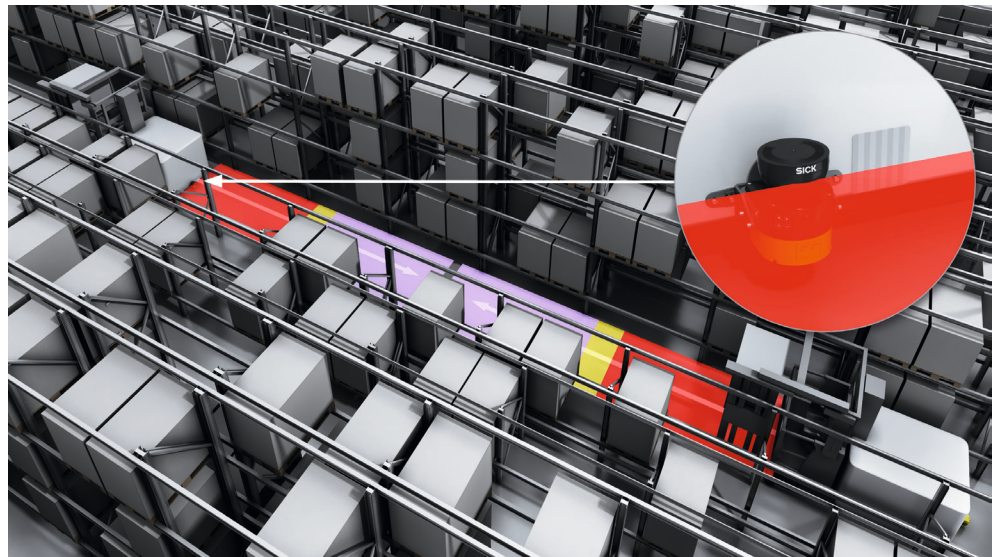
Figure 8: Collision protection field, shown in purple in this document, with reference target, protective field and warning field
