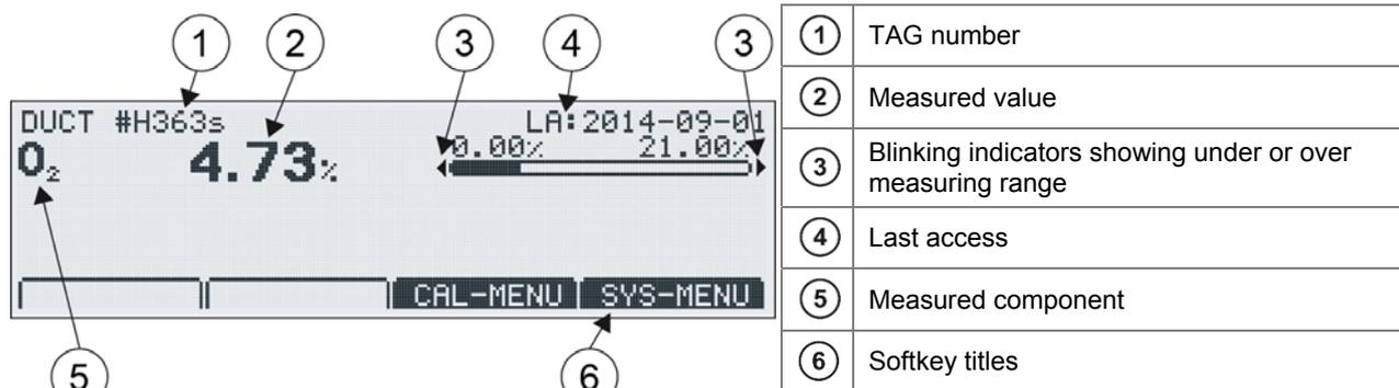
Figure 17 - Measuring mode
