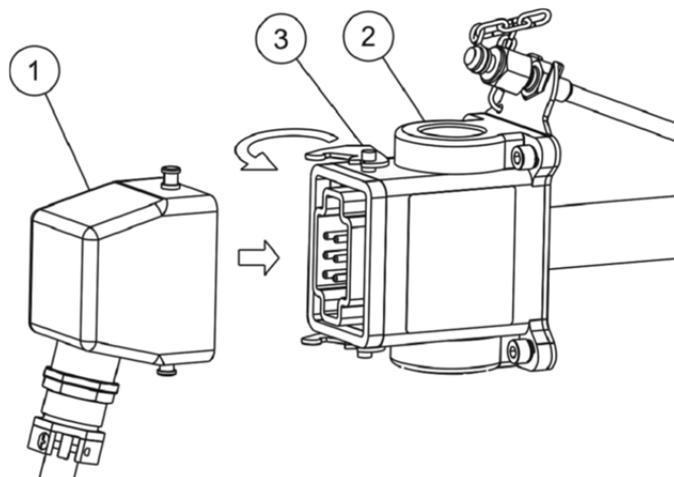
O<sub>2</sub> Probe plug ① has to be inserted into the probe socket ② and locked with the retaining clip ③.
