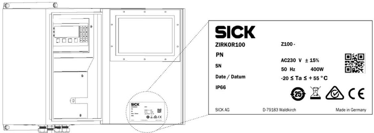
Figure 3 - Name Plate Electronic Unit
