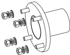
Figure 42 - Duct flange
