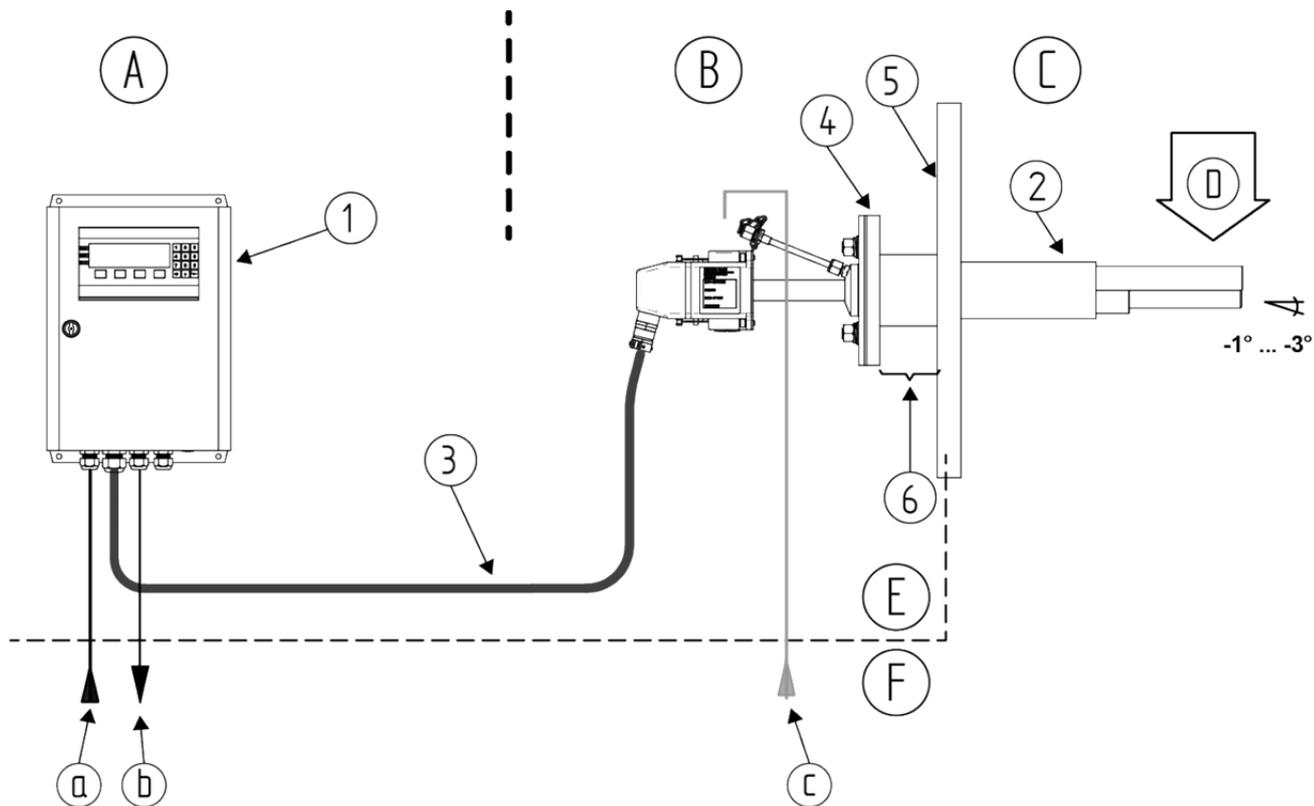
Figure 1 – ZIRKOR100 system (for flue gas temperatures of up to 400°C)
