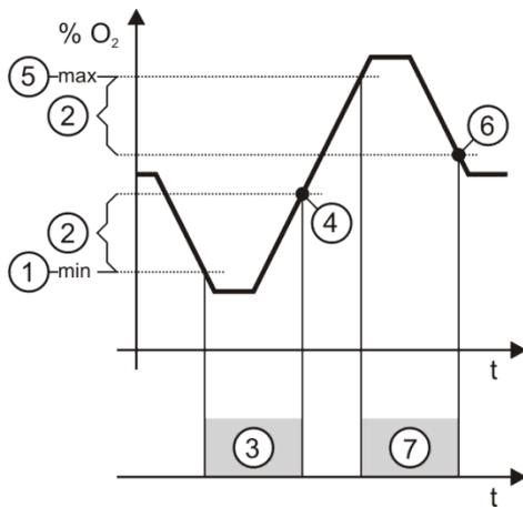
Figure 20 - O<sub>2</sub> limit alarm settings
