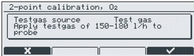
Check and confirm test air/ test gas flow rate before commencing with the calibration
