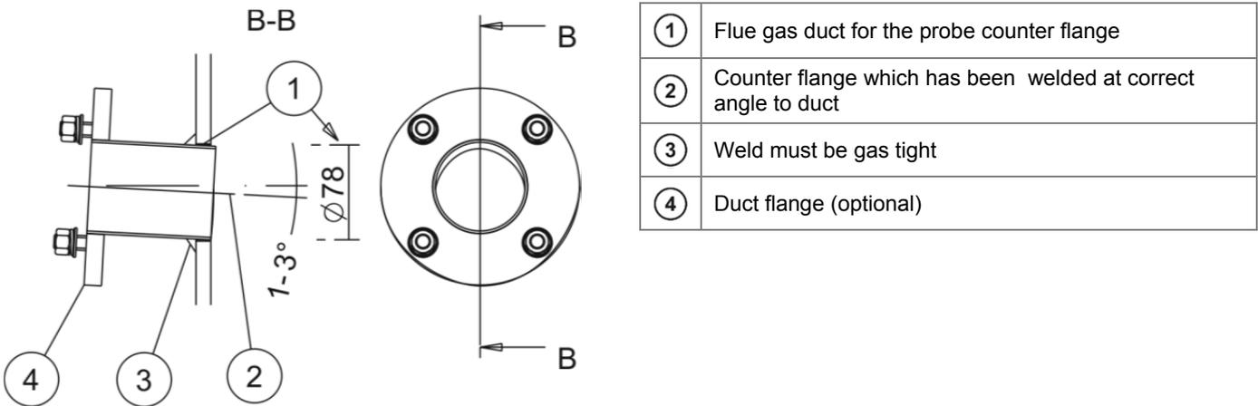
Figure 10 - Welding of duct flange
