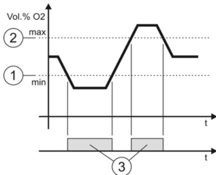
The option O<sub>2</sub> limit alarms observes if the actual O<sub>2</sub> Values are above or below of the adjusted O<sub>2</sub> limits.
