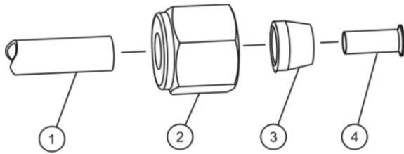
Preparation of the test gas tubing prior to the connection to the O<sub>2</sub> Probe:
