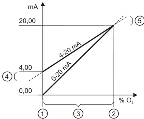
Figure 19 - O<sub>2</sub> Measuring Ranges
