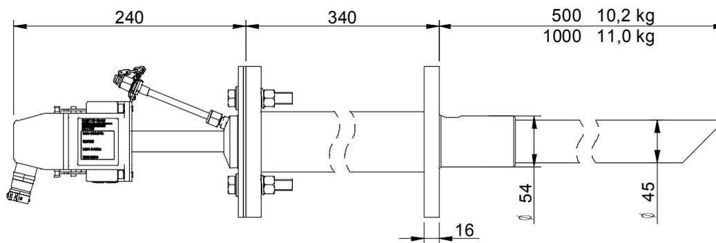
Figure 31 - Low Dust Probe (max. 1400°C)
