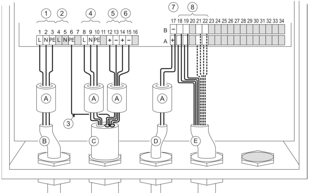
**Figure 8 - Electrical connections of the electronic unit**
