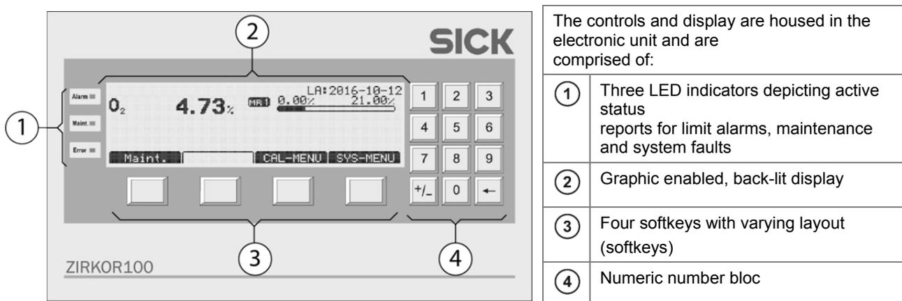
Figure 18 - Keypad and display
