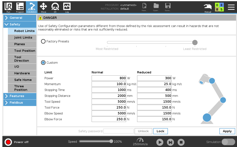
Figure 13: Configuration of stopping times in the robot controller
