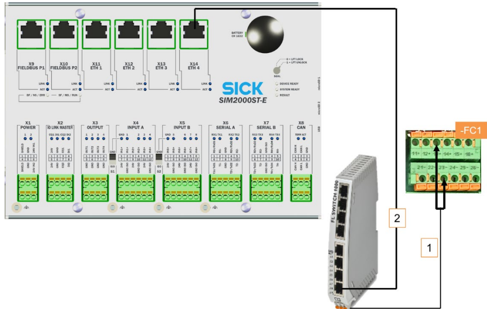
Fig. 84: Connection for LFT Ethernet switch (set up at the factory)
