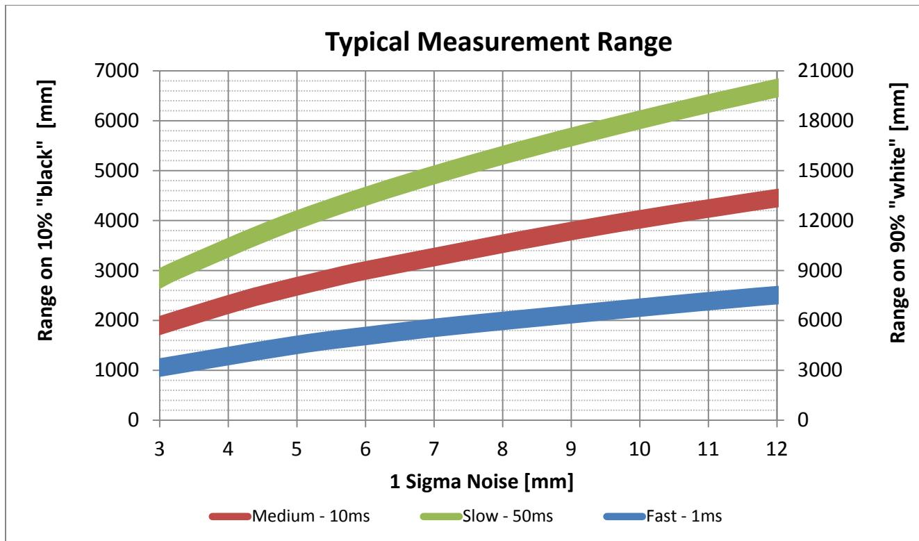
The diagram shows the typical reachable distances over measurement noise. The different colors represent the available measurement profiles.
