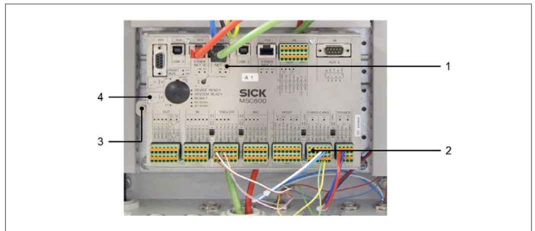
Fig. 53: Unplugging the cables and terminal blocks from the controller
