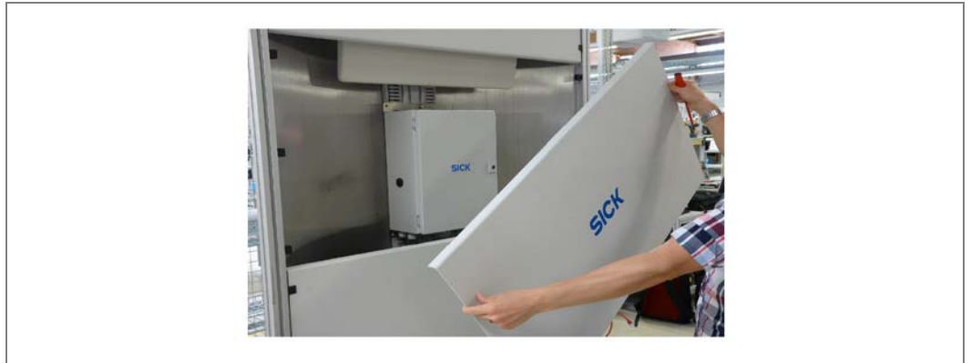
Fig. 51: Securing the cover plate to the side panel
