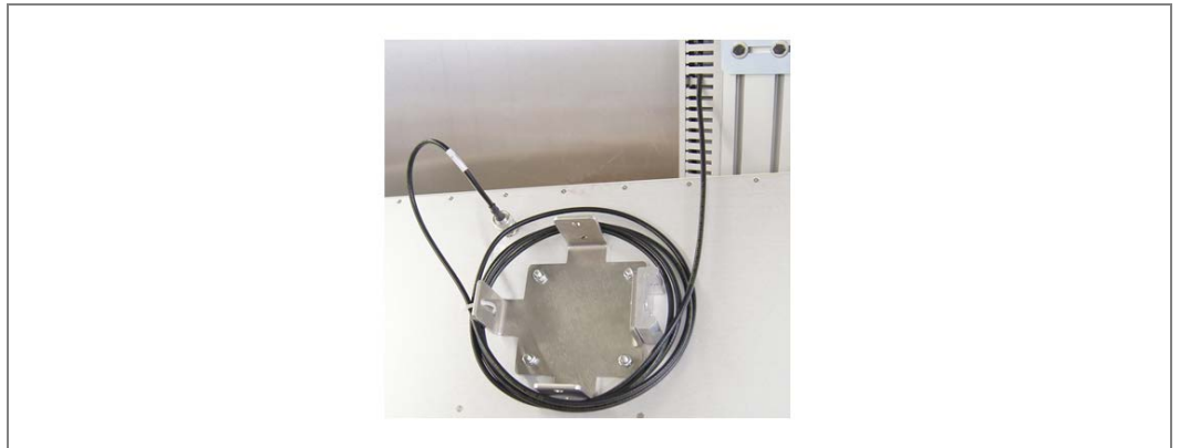
Fig. 46: Winding up excess antenna downloads on the back of the antenna
