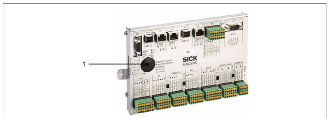
Fig. 54: Position of the battery in the MSC800 controller
