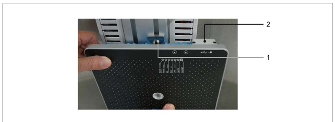
Fig. 58: Removing the interrogator from the mounting rail
