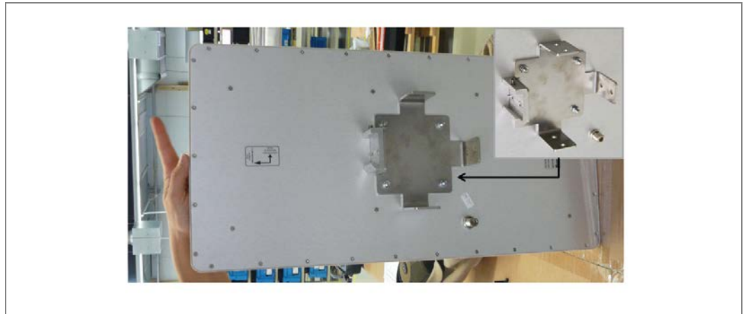
Fig. 59: Mounting the bracket from the defective antenna to the new antenna
