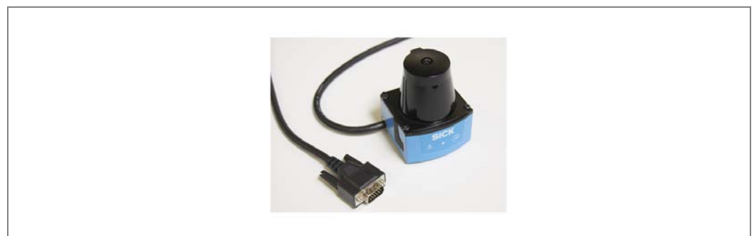
Fig. 39: TiM32x connection to the controller
