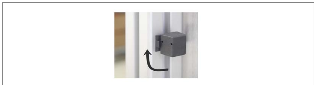
Fig. 50: Swiveling the clamp multiblock in to the profile slot of the side panel
