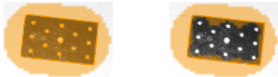
Figure 23: Left image: Creating a part shape region over the entire part. Right image: Using the eraser to exclude holes from the part shape region.
