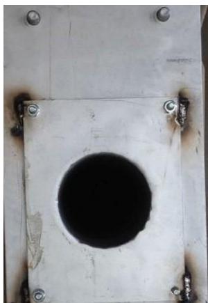
Fig. 22: Protection tube flange plate welded with mounting plate
