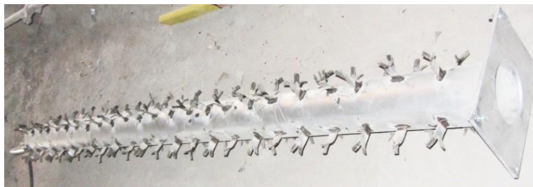
Fig. 21: Protection tube with welded anchoring metal pieces
