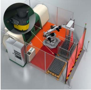
**Access protection at a robot cell**
