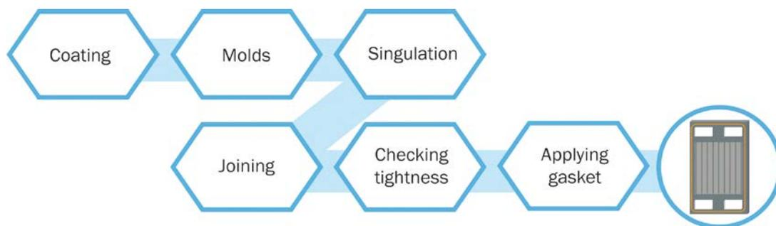
Gas flow, current collection and thermal management of the cell take place in the bipolar plates (BPP). In applications where weight, volume and cost play a major role – as is the case in the automotive industry – BPPs are made of metallic materials. Otherwise, graphite can be used. The manufacturing process is subject to tight tolerances. Due to the several hundred cells that are installed within a stack, even small errors in the flatness and parallelism of the boards lead to large deviations.
