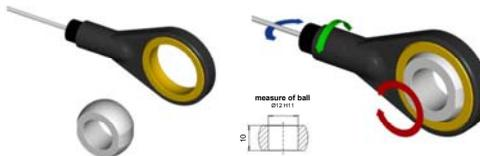
The retrofit built-in of a ball joint in the wire end ring facilitate a movement in different directions.
