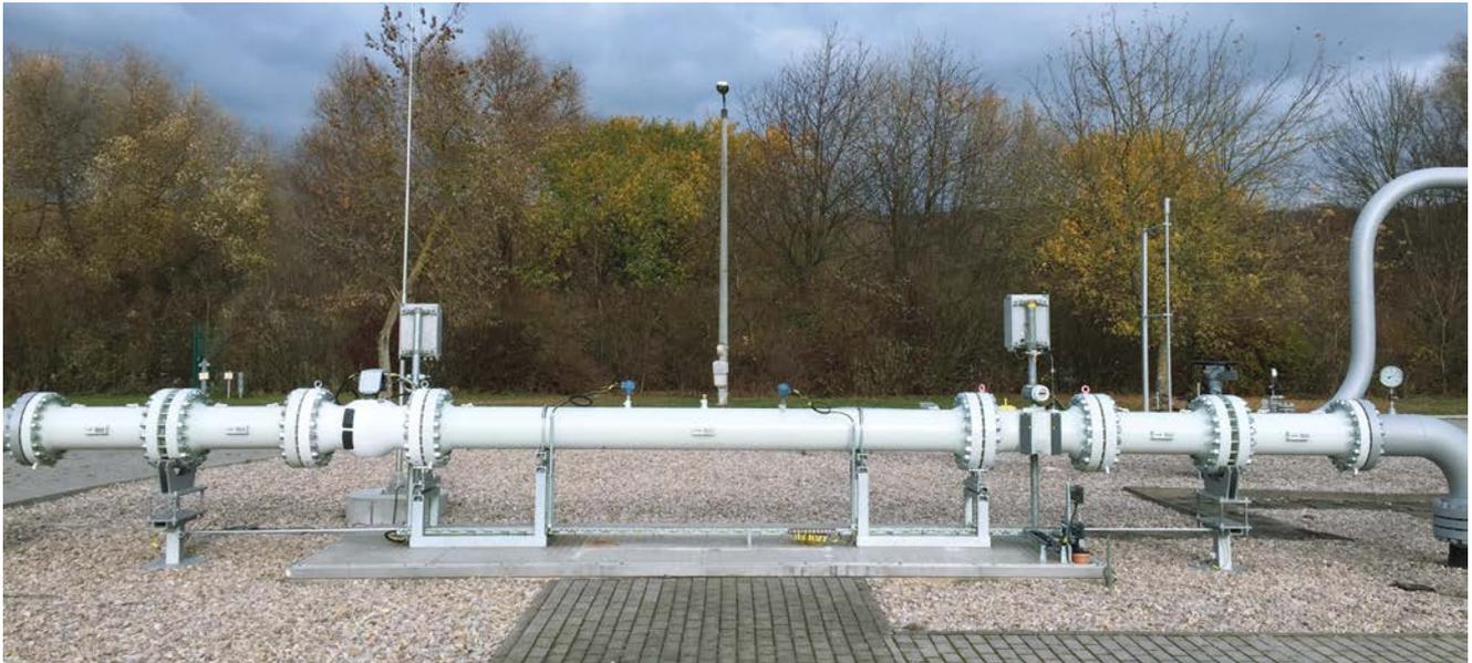
Figure 10: Field test with FLOWSIC600-XT, investigating CBI
