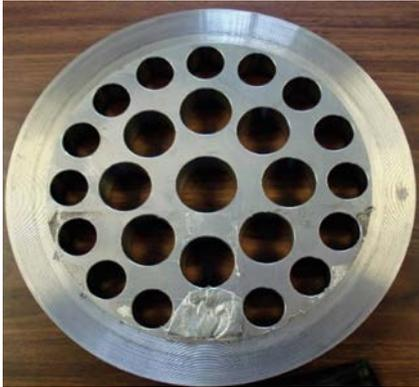
Here too, it was found that the comparison of the 1-path measurement to the 4-path measurement reveals significant deviations before the measurement of the calibrated measurement is influenced. Blockage of even one hole in the flow conditioner plate allows the system to determine a relative deviation of the 1-path system of up to -0.85%, while the 4-path system continues to measure with a high level of accuracy (see diagrams 4 and 5).
