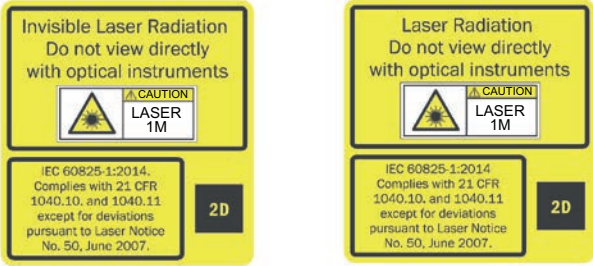
Fig. 1: Warning symbol on the device LASER RADIATION Do not view directly with optical instruments. Class 1M laser product
