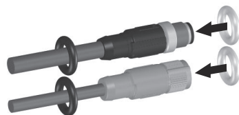
Figure 12: Assembly of IP69K protective housing, with use of the Ethernet connection – Step 1
