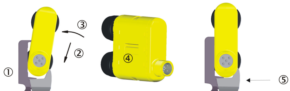
Figure 37: Mounting the Flexi Loop node using a C-Fix bracket
