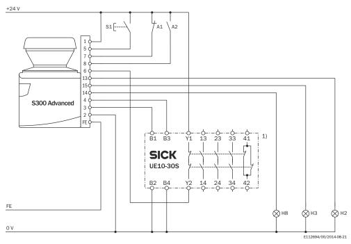
Figure 40: Connection diagram for monitoring case switching using one static input pair
