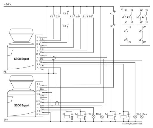
Figure 43: Connection diagram for monitoring case switching between two safety laser scanners with static inputs
