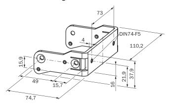
Figure 87: Dimensional drawing mounting kit 1a (mm)
