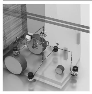
Figure 72: Example for speed routing on an AGV
