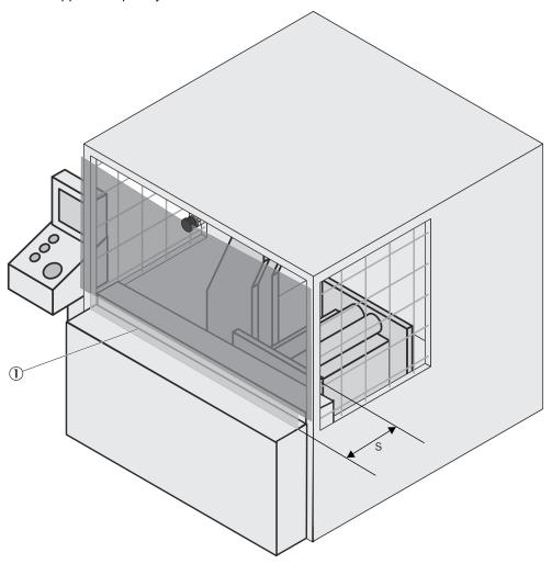
Figure 33: Minimum distance to hazardous area
