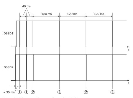
Figure 81: Diagram of the test pulse at the OSSDs
