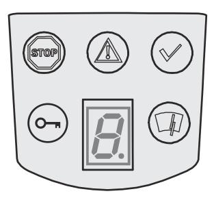
Figure 6: Status indicators of the safety laser scanner
