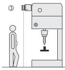
Figure 65: Schematic representation of operation with restart interlock
