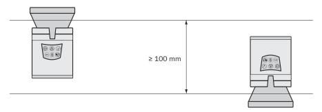
Figure 21: Mounting one device upside down, offset parallel
