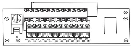
Figure 52: Screw terminal block of the system plug
