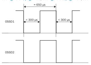
Figure 82: Voltage test after switching on the OSSDs
