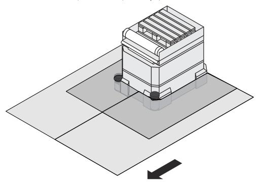
Figure 24: Mounting example for front and side protection in one direction of travel
