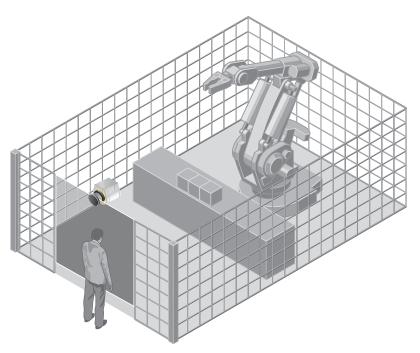
Figure 13: Access protection: detection of a person when accessing a hazardous area
