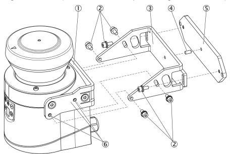
Figure 51: Mounting using mounting kit 2
