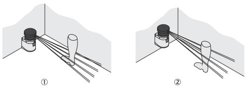
Figure 31: Relationship between resolution and protective field mounting height
