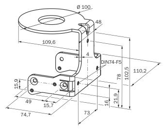
Figure 88: Dimensional drawing mounting kit 1b (mm)
