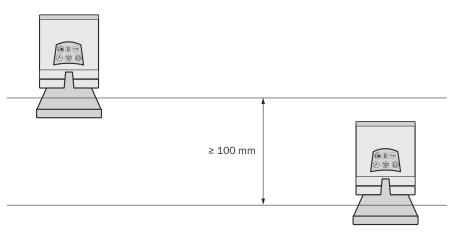
Figure 20: Mounting both devices upside down, offset parallel
