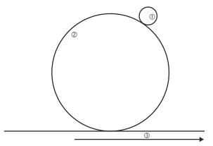
Figure 62: Calculation of pulses per cm travel
