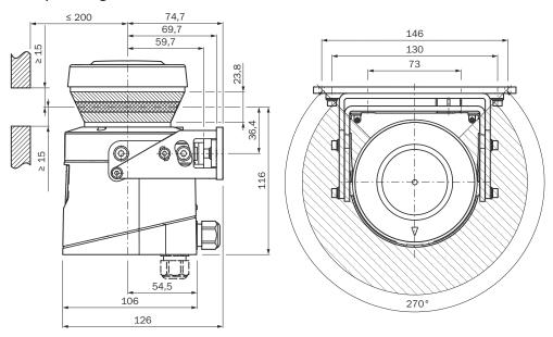
Figure 86: Dimensional drawing scan plane origin with mounting kit 1a, 2 and 3 (mm)
