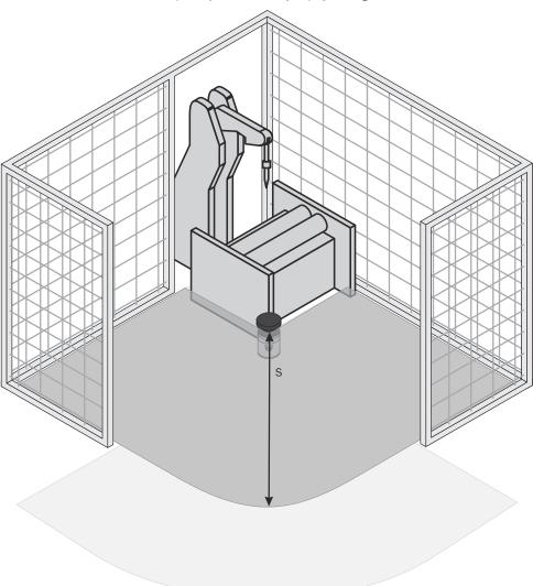
Figure 28: Horizontally mounted stationary application
