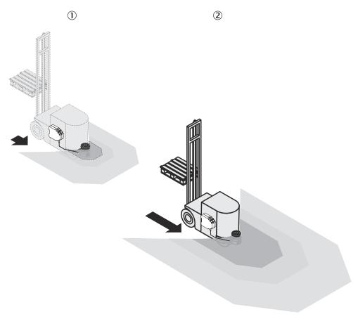
Figure 8: Safety laser scanner with two monitoring cases on one AGV
