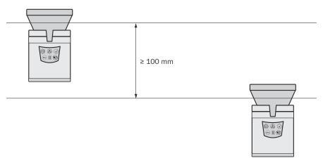
Figure 17: Mounting offset parallel
