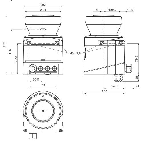
Figure 85: Dimensional drawing safety laser scanner (mm)
