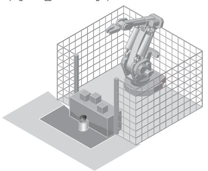
Figure 11: Hazardous area protection: detection of the presence of a person in the hazardous area
