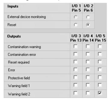
Figure 66: Configuration example for universal I/O connections
