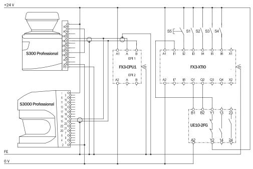
Figure 46: Connection diagram for monitoring case switching between S3000 and S300 usin a Flexi Soft safety controller
