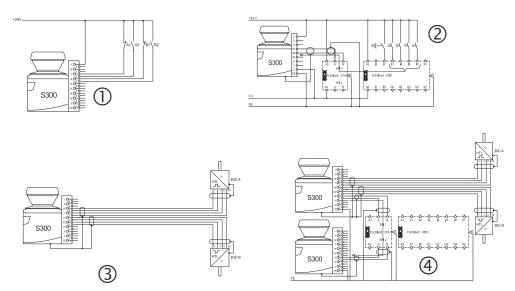
Figure 64: Possible ways of monitoring case switching
