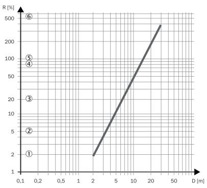
Figure 79: Diagram scanning range with Medium Range
