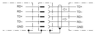
Figure 53: Connection diagram for the RS-422 interface
