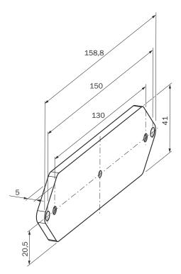
Figure 90: Dimensional drawing mounting kit 3 (mm)
