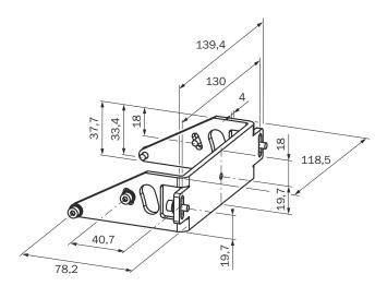
Figure 89: Dimensional drawing mounting kit 2 (mm)
