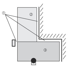
Figure 68: Configuring the protective field and warning field
