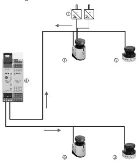
Figure 73: Connection diagram for speed routing
