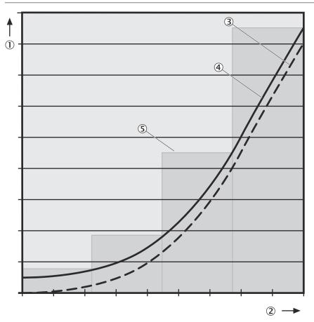
Figure 35: Stopping distance as a function of the vehicle's speed
