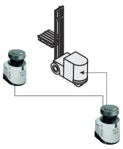
Figure 10: EFI system with safety laser scanner
