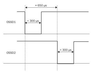
Figure 83: Shut-down test
