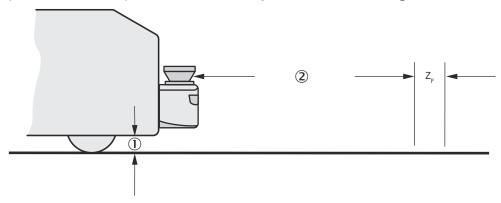
Figure 36: Supplement due to lack of ground clearance
