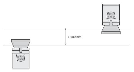
Figure 19: Mounting upside down, offset parallel
