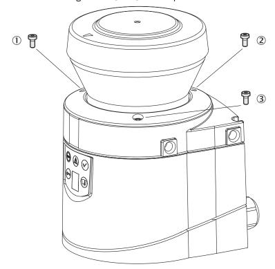
Figure 78: Remove the fixing screws of the optics cover
