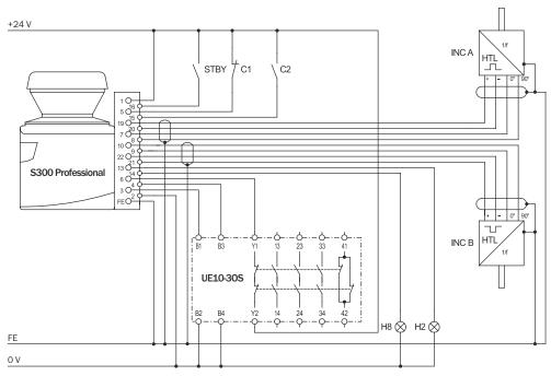
Figure 42: Connection diagram for monitoring case switching using static and dynamic inputs
