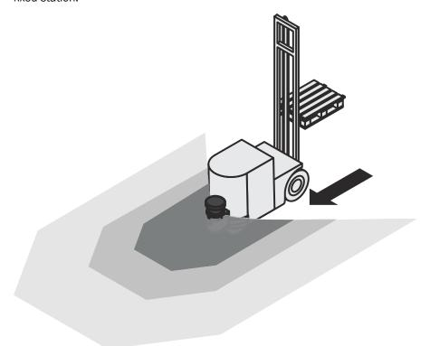
Figure 14: Mobile hazardous area protection: detection of a person when a vehicle approaches
