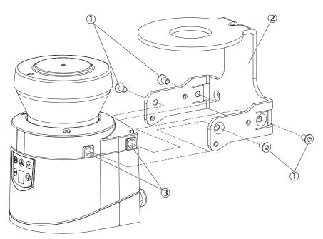
Figure 50: Mounting using mounting kit 1b including optics cover protection
