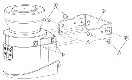
Figure 49: Mounting using mounting kit 1a
