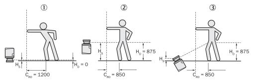
Figure 30: Mounting options for the scan plane
