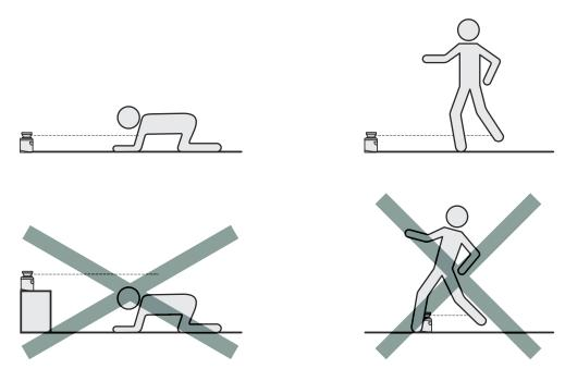
Figure 15: Prevent crawling beneath, standing behind, or climbing over
