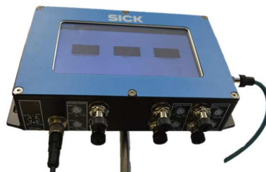
Fig. 52: Replacing components – Display (removing the cables)
