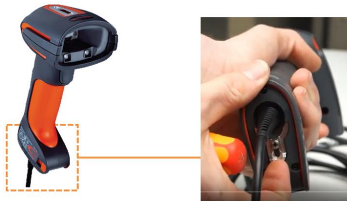
Fig. 51: Replacing components – Hand-held scanner
