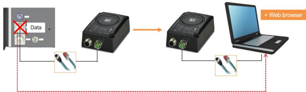
Fig. 39: Connecting the configuration PC to the WLAN module
