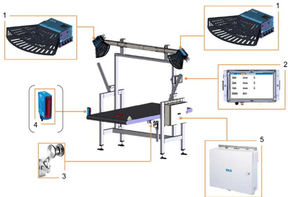
Fig. 1: Components of the VMS4200/5200(Multicontroller)
