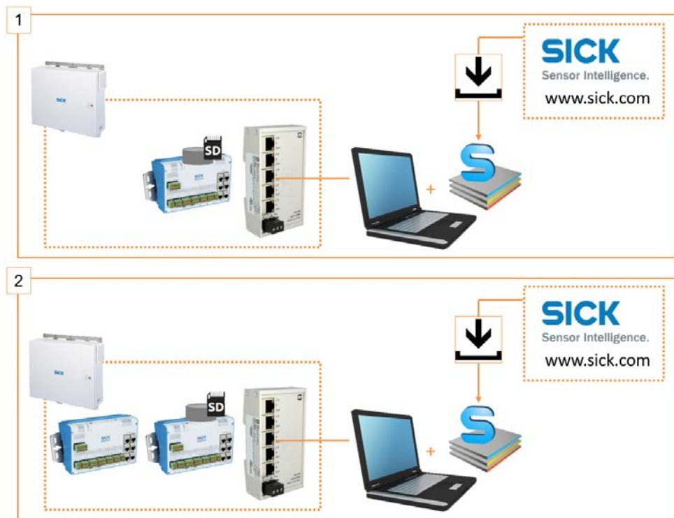
Fig. 74: Establishing the configuration PC - SIM2000 system controller connection
