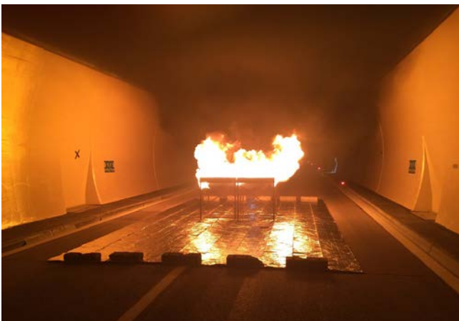
Image 5: Fire and smoke development during a fire test
