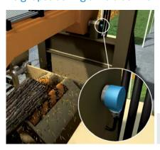
The height of the hold-down arm is detected with the ATM60 position encoder for determining the log diameter. The rotation time is calculated from this.
