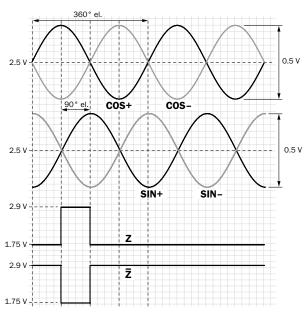
Interface signals Sin+, SIN-, COS+, COS- Signals before difference at 120  $\Omega$  load Signal offset Differential analog 0.5  $V_{SS} \pm 20\%$  2.5  $V \pm 10\%$
