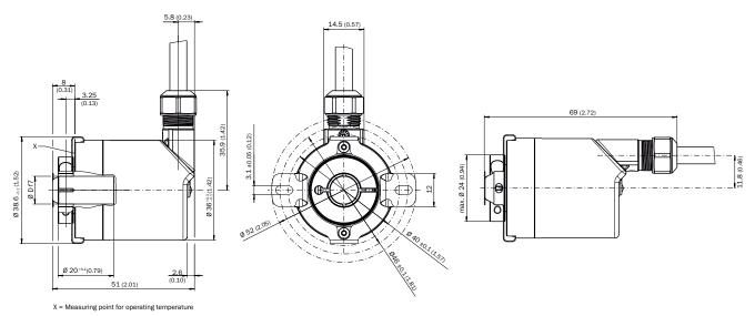
Bend radius of cable; R = 30 mm
