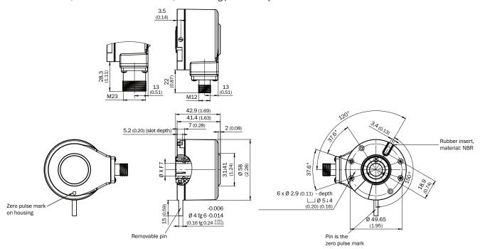
Installation example for blind hollow shaft
