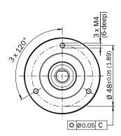
General tolerances according to DIN ISO 2768-mk 1 Cable  $\varnothing$  = 5.6 mm  $\pm$  0.2 mm bend radius R = 30 mm
