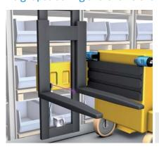
Using a BKS09 wire draw encoder enables the narrow aisle truck to accurately determine the position of the fork. The highly flexible steel wire is fixed to the
