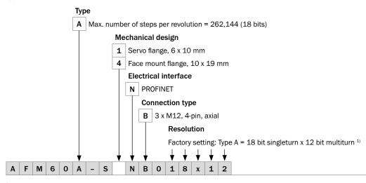
$<sup>^{\</sup>mbox{\tiny 1)}}$  Programmable options for resolution via control unit.
