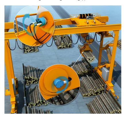
When moving and loading logs using cranes, you must be able to detect the height of the gripper. An absolute encoder mounted on the drum is ideal for this purpose. An additional absolute encoder is mounted on the gripper itself to calculate the opening angle in use.
