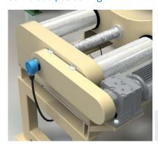
The positioning of saw-blades for setting to the thickness to be sawed is carried out with the ATM60 absolute encoder.
