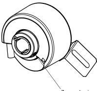
Zero pulse is active when screw of clamping is in line with zero pulse mark on flange or housing mark
