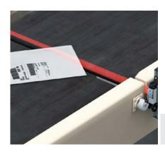
The leading edge detection serves to convey objects at a specified distance from the belts to the main sorter. The combination of high-resolution light grids and high-resolution encoders allows leading edge detection and the detection of additional object profile information such as the length.
