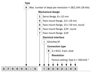
$<sup>^{1)}</sup>$  Number of steps programmable via control unit: Type A = 2 to 262144.
