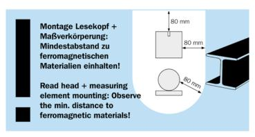
Only use non ferro-magnetic materials for the assembly base of the read head. A separation distance of 80 mm must be observed for ferro-magnetic materials (e.g., iron).
