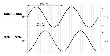
Incremental signal outputs for clockwise shaft rotation, looking in direction "A" (see dimensional drawing)
