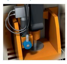
Once the tools have been replaced, the press stroke must be adapted using a primarily mechanical adjustment mechanism. The procedure for adjusting the height of the press stroke can be
