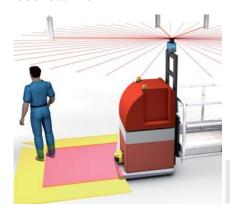
For personal protection and collision prevention with other vehicles or materials on the floor, automated guided systems AGS are equipped on the fork side and on the back side with safety laser scanners. The AGS is equipped with two drive units with one DBS60 Core incremental
