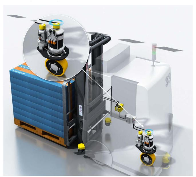
The safety encoder provides information on the speed and rotational direction of the driver and thus on the speed and direction of the automated guided system.
