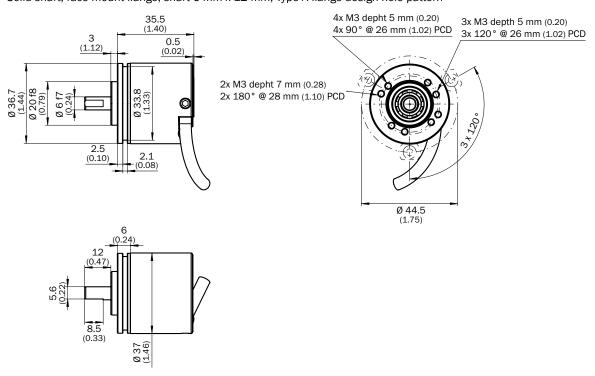
Solid shaft, face mount flange, shaft 1/4" x 15.5 mm, standard hole pattern
