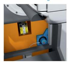
The BCG08 EcoLine wire draw encoder determines the fork lifting height of the automated guided system and forwards this to the vehicle controller. The BCG08
