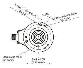
Solid shaft Ø 6 mm, face mount flange, male connector connection (S3)
