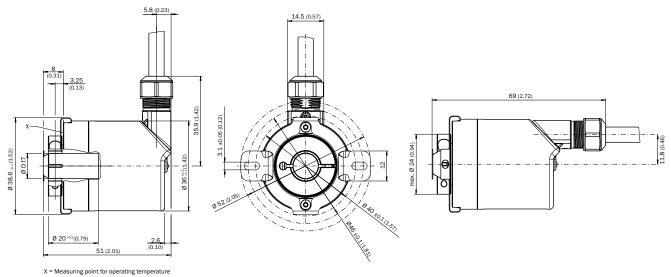
Bend radius of cable; R = 30 mm
