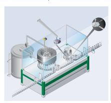
The precise position and speed monitoring is handled by an A3M60 absolute encoder. The encoder is connected directly to the carousel wheel via gear stages. The resolution per rotation depends on the number of filling stations. The number of encoder rotations depends on
