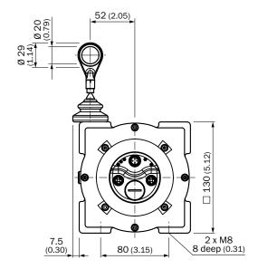
BTF13 up to 10 m EtherNet/IP, EtherCAT®, PROFINET
