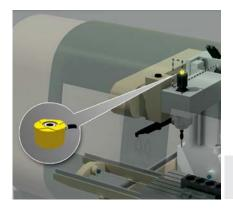
For stand-alone machines such as a drilling machine, the user is protected from the hazardous point by a safety door or hood. For set-up operation, the speed of the drilling arm and tool table must be
