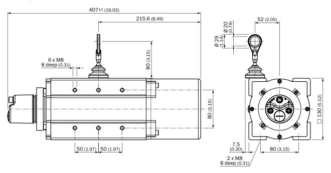
BTF19 up to 50 m EtherNet/IP, EtherCAT®, PROFINET
