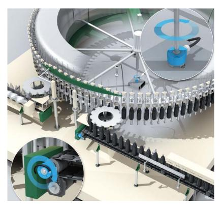
In the bottling line shown here, bottles are collected in the rotating turntable filling stations from the left-hand side and are filled as they rotate. Once full, the bottles are placed on a conveyor belt. The position and speed of the rotating turntable and the conveyor belt are monitored using an absolute encoder.
