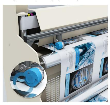
Incremental encoders detect the speed of the print media and provide key information on the correct position for the print and the quality of the printed image. Whether you require clearly legible bar codes or high resolution printed check cards, gift cards, or brochures – accurate speed monitoring ensures print quality.
