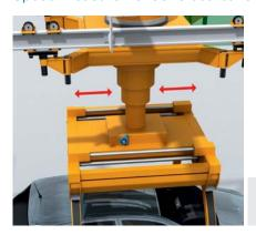
The electrical overhead conveyor brings the car bodies to designated workplaces. The speed is specified by the higher-level control; an incremental encoder determines the speed. In case of requirements for secure speed, the DFS60S Pro assists with the realization of collision protection in combination with a safety laser scanner.
