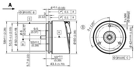
General tolerances according to DIN ISO 2768-mk 1 Cable Ø = 5.6 mm  $\pm$  0.2 mm bend radius R = 30 mm
