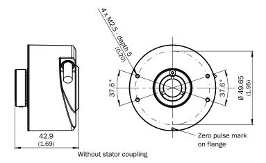
Installation example for blind hollow shaft
