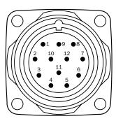
View of 12-pin M23 device connector on SSI encoder
