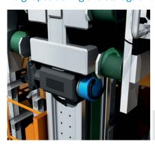
When it comes to the insertion depth, accurate measurements are crucial. A rugged absolute encoder on the belt drive with a high resolution and excel-
