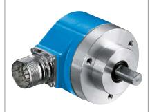
The ATM60 absolute multiturn encoder from SICK has an SSI data interface and provides reliable positional information even in harsh ambient conditions, with a resolution of up to 26 bits. This product family, which is proven in its field, is based on the principle of magnetic measurement. The 13 bit singleturn range is scanned by a sensor using permanent magnetic elements. The 13 bit multiturn
