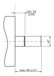
General tolerances according to DIN ISO 2768-mk  $x_j$ 7 = Shaft diameter, on the customer side
