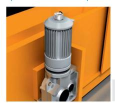
The DFS60 incremental encoder supplies the value for controlling the positioning speed, acceleration, and delay. On entry into the protected area of the storage and retrieval system, it must
