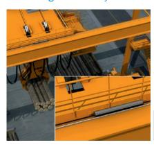
The KH53 is ideally-suited for positioning the trolley on the crane thanks to its good repeatability, large reading distances, and outstanding robustness in case of shocks, vibrations, and weather
