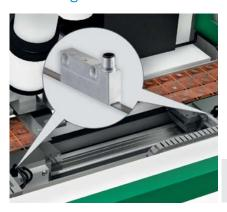
Temperatures are very high in the area around the bonding head, making fiber-optic cable systems the most effective for this application. With its 16  $\mu s$  response time, the WLL180T works together with the LL3-TH fibers to supply the control unit with a precise signal for edge detection. The grippers of the wire
