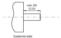
Through hollow shaft clamping at the back, male connector connection, no stator coupling
