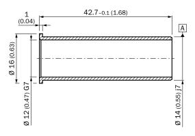
PEEK conductor insulation, 12.7 x 15 mm
