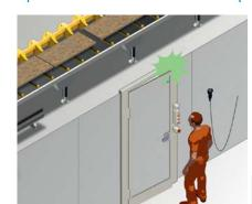
On the saw line, the operator is kept away from the hazardous point by a safety fence. In order to eliminate faults on the line, a safe standstill detection is necessary or for the maintenance and
