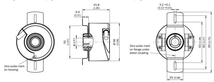
Installation example for through hollow shaft
