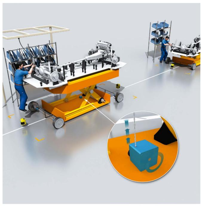
Scissor lifts are used, for example, in the automotive industry for vehicle assembly. It is important that the scissor lifts are at the ideal working height for the operators.
