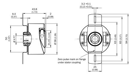
Installation example for blind hollow shaft
