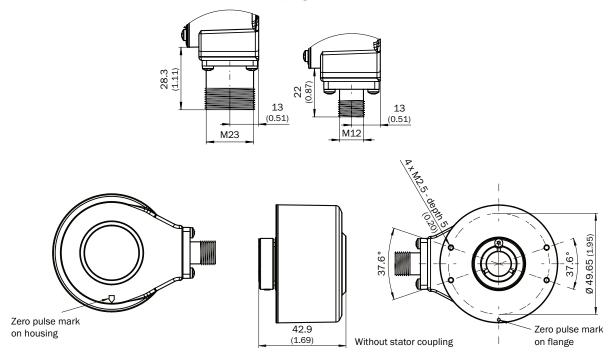
Blind hollow shaft, male connector connection, with locating pin assembly
