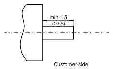
Through hollow shaft, cable connection, stator coupling, 1-sided, slot, bolt circle 33 mm - 48.5 mm
