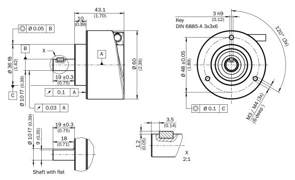
General tolerances according to DIN ISO 2768-mk Cable diameter =  $5.6\pm0.2$  mm; R bend radius = min. 7.5 x cable outer diameter
