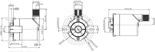
X = Measuring point for operating temperature
