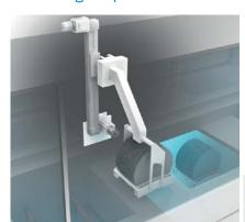
The position of the wafer carrier is determined reliably with absolute encoders: with the AFS60 Singleturn on the vertical and the AFM60 Multiturn on the hori-
