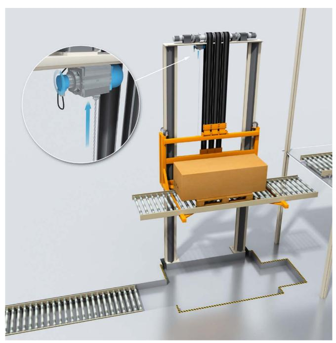
Within logistics processes, such as in the automotive industry, levels often have to be passed over to continue to convey goods. Lifts are used for this purpose, and their platforms must be accurately positioned flush to the target level.
