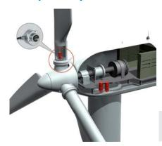
The adjustment of the rotor blades plays an important role in order to achieve as great a yield as possible of rotation energy. Depending on the wind strength and direction, the position of the rotor blades is adjusted accordingly. AFS60/AFM60 absolute encoders are used to set the
