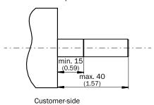
Blind hollow shaft, male connector connection, stator coupling, 1-sided, slot, bolt circle 33 mm - 48.5 mm
