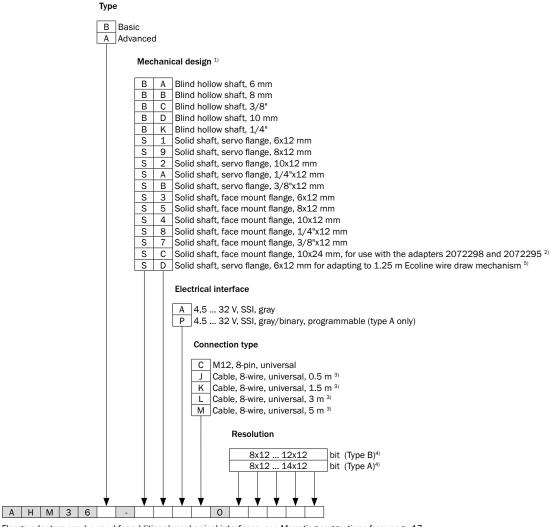
$<sup>^{1)}</sup>$  Flange adapters can be used for additional mechanical interfaces, see Mounting suggestions from page 17.
