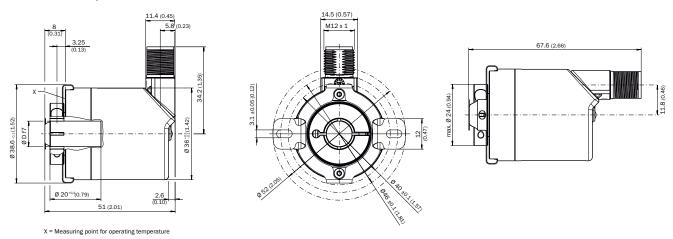
Customer's own shaft: insertion depth of at least 15 mm to max. of 22 mm, from contact surface, from stator coupling, recommended shaft tolerance of k7
