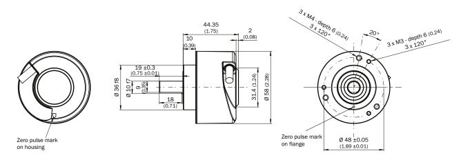
Solid shaft Ø 6 mm, face mount flange, cable connection (S3)
