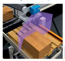
With both laser measurement and absolute encoders, an image and a position of the load can be determined, enabling
