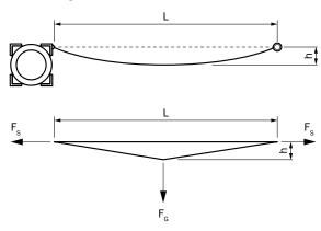
The weight-related force of the measuring wire can be calculated using Formula A.
