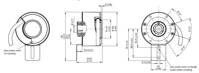
Installation example for blind hollow shaft
