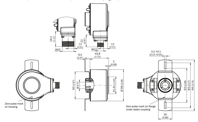
Blind hollow shaft, male connector connection, no stator coupling
