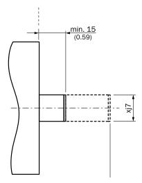
General tolerances according to DIN ISO 2768-mk xj7 = Shaft diameter, on the customer side
