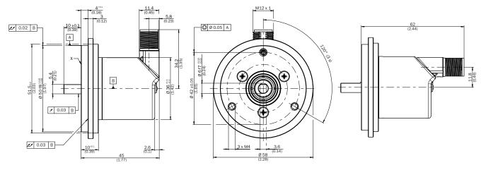
X = Measuring point for operating temperature
