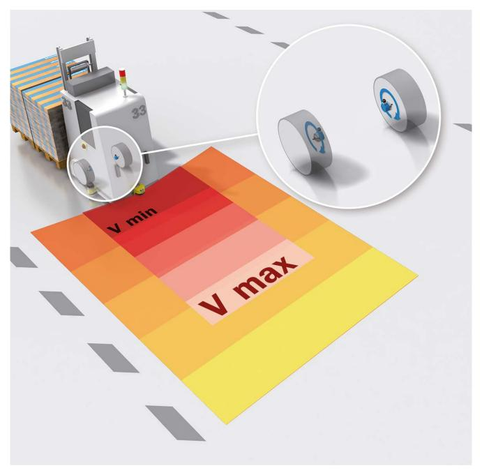
The incremental encoder provides information on the direction of travel and the speed of the automated guided system (AGS). The encoder can either be directly mounted on the motor, on an axle (see figure), or on a revolving wheel.
