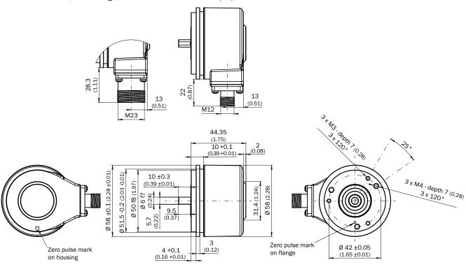
Solid shaft  $\emptyset$  6 mm, servo flange, cable connection
