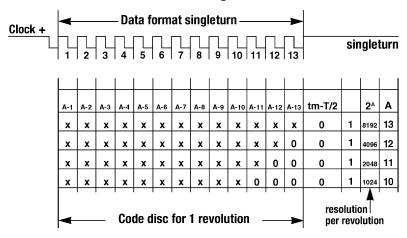
SSI data format for resolutions > 8,192 (14 and 15 bit)
