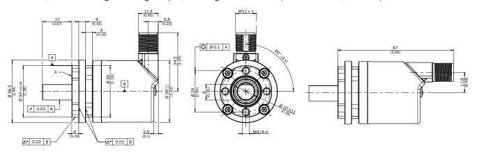
X = Measuring point for operating temperature
