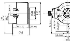
Installation example for blind hollow shaft
