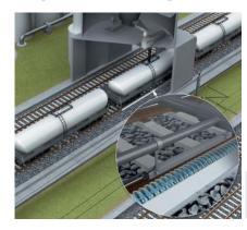
So that loading and unloading is completed correctly, especially with automatic systems, freight trains must be positioned exactly. With a measurement length of max. 1,700 m, the KH53 linear encoder is especially well-suited for use
