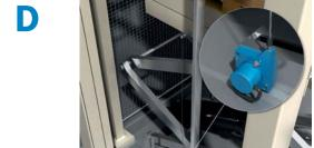
The scissor lift table is positioned using a high-resolution wire draw encoder with a teach-in function. The extremely reliable wire draw encoder does not require complex linear guidance, and can be integrated with ease both electrically and mechanically.
