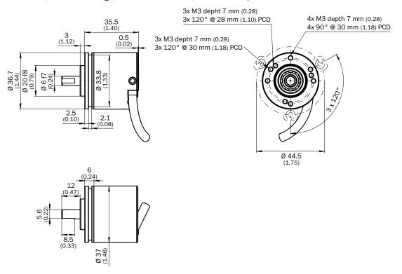
Solid shaft, face mount flange, shaft 6 mm x 12 mm, Type A flange design hole pattern
