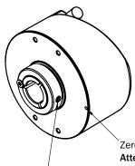
Zero pulse is active when screw of clamping is in line with zero pulse mark on flange or housing mark Zero pulse mark on flange Attention!
