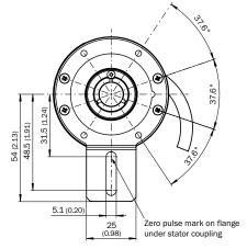
Installation example for through hollow shaft
