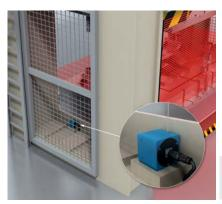
To determine the position of the press stroke, a BKS wire draw encoder is used. It reliably supplies signals for establishing the top dead center (TDC) and bottom dead center (BDC).
