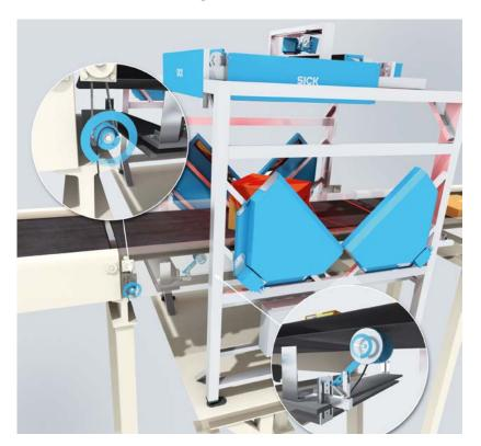
The incremental encoder detects the speed of the conveyor belt and the objects transported on it. Using this information, the speed of other conveyor belts can be synchronized – for example, to control bar code scanners and label printers.
