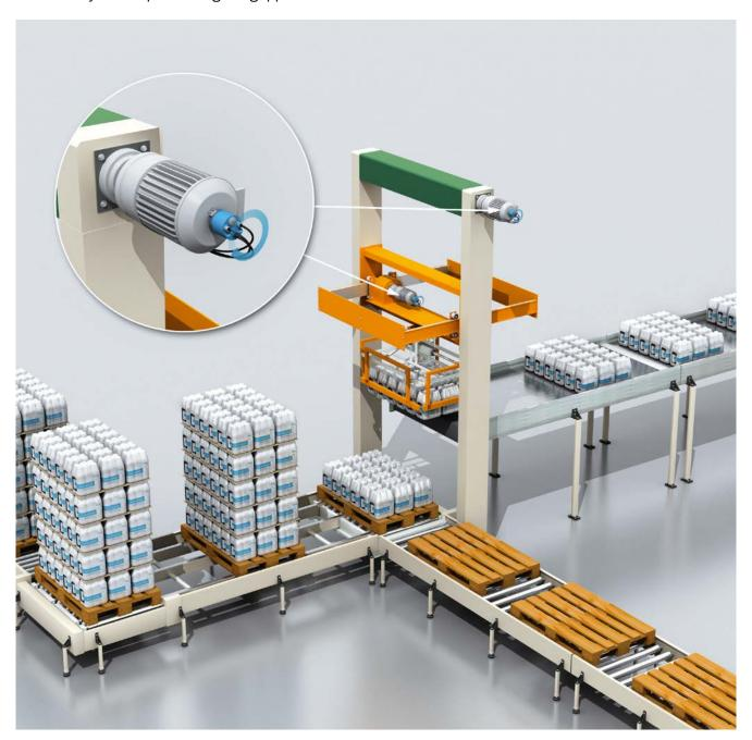
For example, plastic bottles are stacked in multiple layers on pallets in a palletizer system. The gripper of the pallet handling machine must be positioned in the X and Y directions. An absolute encoder is used to determine the position of the gripper.
