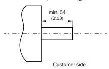
Through hollow shaft clamping at the back, cable connection, no stator coupling
