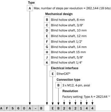
$<sup>^{1)}</sup>$  Number of steps programmable via control unit: Type A = 2 to 262144.
