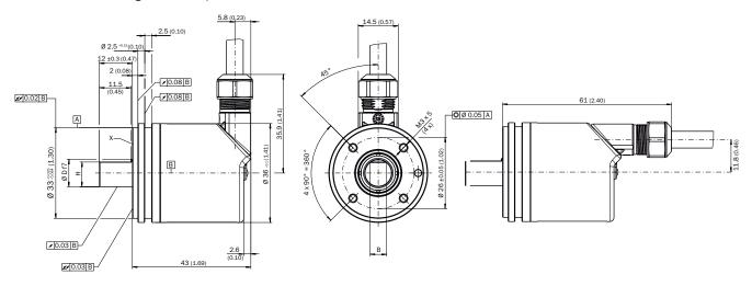
X = Measuring point for operating temperature
