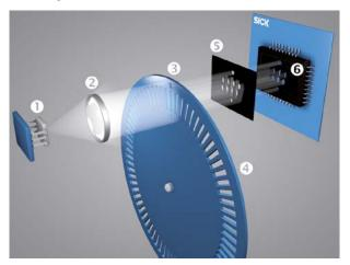
1 LED; 2 Lens; 3 Reference point; 4 Code disc; 5 Mask; 6 Photo-diode.
