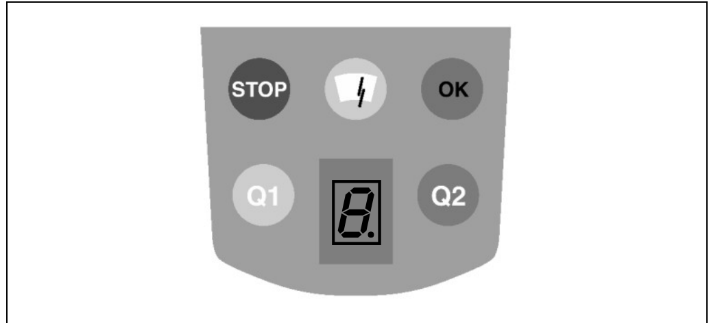
Fig. 48: Status indicators of the LMS80-S01
