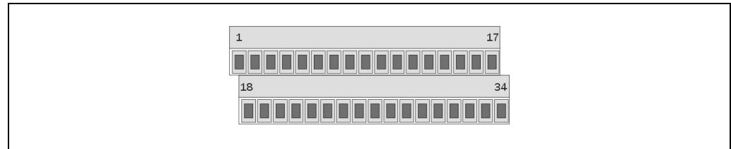
Fig. 36: 34-pin screw type terminal for the LMS80-S01
